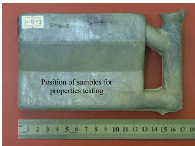
Fig. 1 Casting with the fabricated area of the samples for the mechanical properties tests
